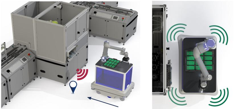
(a) The assembly module sends a signal, which the LH6 responds by arriving to a given destination.
