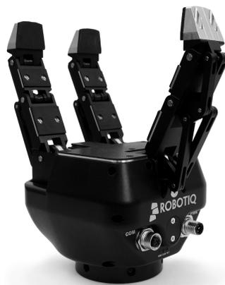
Figure 6.4: Robotiq 3-Finger. (Universal-Robots-A/S 2016b)
