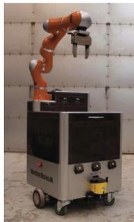
**Figure 1.1:** Illustrates LH3 consisting of a KUKA LWR manipulator, integrated together with at Neobotix mobile platform. (Carøe, Hvilshøj, and Schou 2012)
